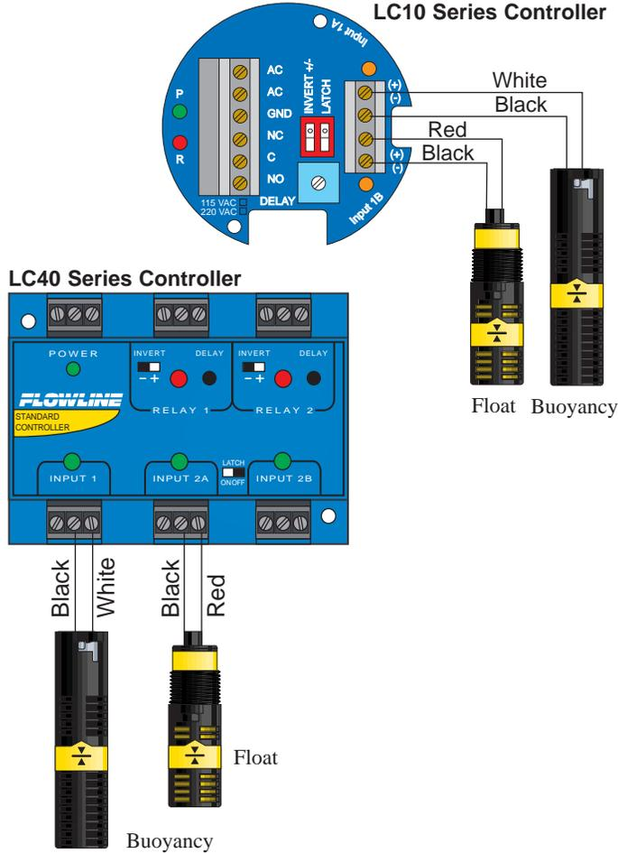
**Note:** Above wiring is for NO operation (open circuit when switch is dry and closed circuit when switch is wet). To wire NC (closed circuit when dry and open circuit when wet), use RED and BLACK wires for the LV10-3\_1 or reverse the float for the LV10-2\_1. Use the shield to protect the cable from electrical noise. Attach to either the Shield terminal or the ground terminal.
