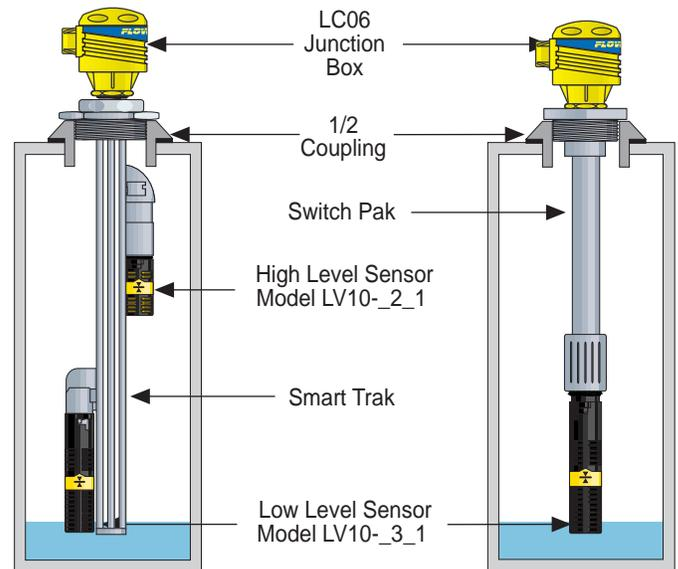
**Note: Avoid installing the LV10 in magnetized metal tanks. Doing so will activate the internal reed switch.**
